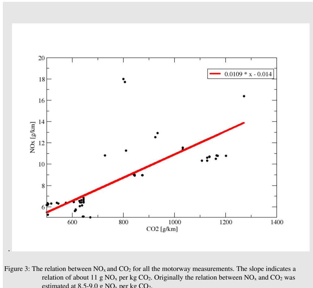
The data shows a relatively consistent picture of 11 grams NO<sub>x</sub> per kg CO<sub>2</sub>, indicated by the line, over the whole range of vehicles mass and payloads, on the motorway. In urban driving circumstances the emission is 13 grams NO<sub>x</sub> per kg CO<sub>2</sub>.
