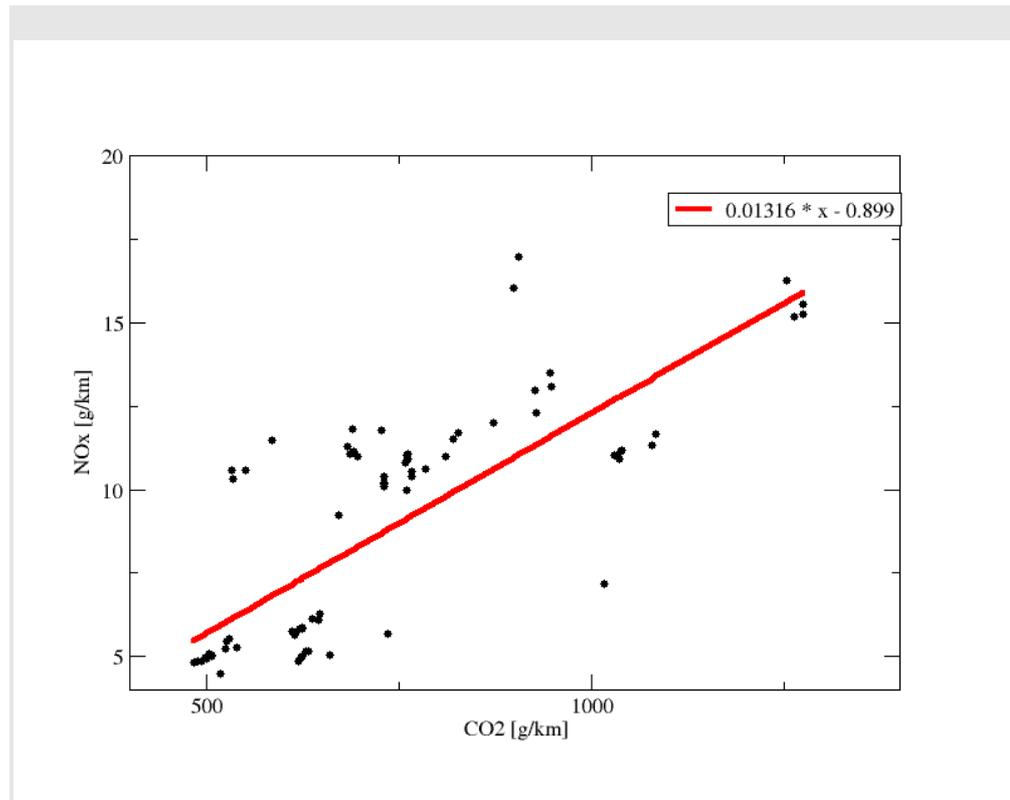
Figure 4: the relation between NO<sub>x</sub> and CO<sub>2</sub> for all the city measurements. The slope indicates a relation of about 13 g NO<sub>x</sub> per kg CO<sub>2</sub>. Originally the relation between NO<sub>x</sub> and CO<sub>2</sub> was estimated at 8.5-9.0g NO<sub>x</sub> per kg CO<sub>2</sub>.
